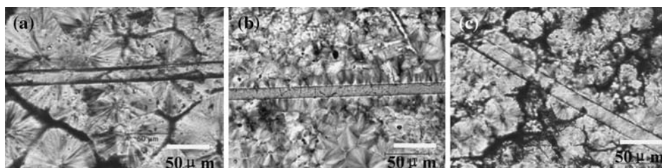
Fig. 7 Photographs of the border in PP/GF modified by different block copolymer coupling agent in isothermal crystallization at 135 °C ( \times 500 ) (a) Sample 4(PP+GF (PS57- b -PMPS27)) (b) Sample
